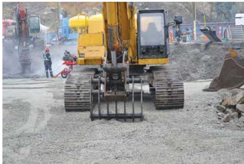
Excavator bucket designed by Allterra to more effectively dig for the types of metal and cabling that crews had to contend with at the FMF Cape Breton site.
